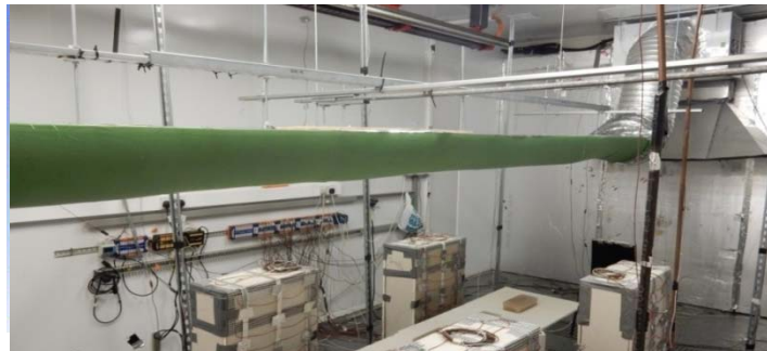
Air distribution system with a half-fabric duct at a medium level
